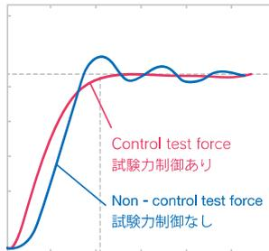
Test force is controllable with high precision from the output of a load cell.
