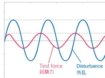
Feedback control controls the vibration from the outside.
